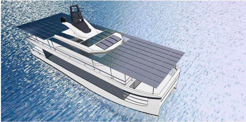
Figure 5-1. Illustration of the 33-m-long twin-hull vessel with integrated solar panels.
