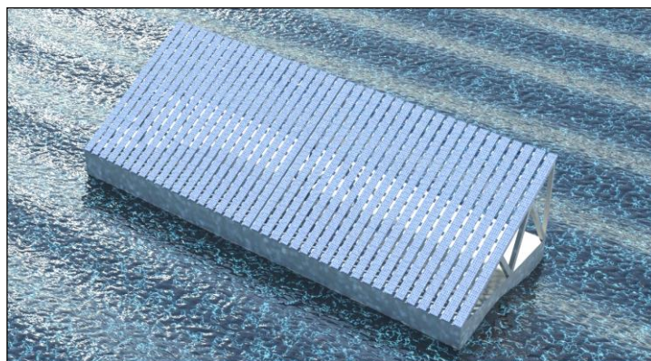
Figure 4-1. Pontoon-type floating structure supporting arrays of photovoltaic panels.
